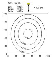
Light sourceLEDWork equipmentWithoutConnected load22 - 26 V; DCPower consumptionca. 32 W
